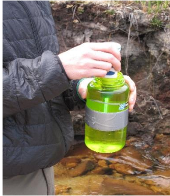
Figure 3 An ultraviolet light water sterilization pen and an ultraviolet light tanning bed both use invisible ultraviolet light to interact with the DNA of living cells.
